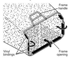
**ACAUTION:** Under normal usage, the catcher material is subject to deterioration and wear and should, therefore, be checked frequently for replacement. Any replacement catcher should be checked to ensure compliance with original manufacturer's specifications.
