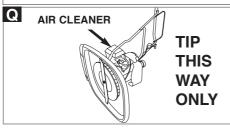
Before any servicing to the underside of your machine, close the fuel tap, let the engine run until it stops, disconnect the spark plug lead and TIP THE MACHINE ON ITS SIDE WITH THE AIR CLEANER **UPPERMOST (Q).**
