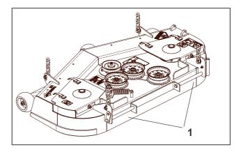
*Tunnel Ram Deck Installation* 1. Strut Pins
