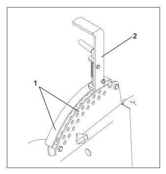
**Deck Lift Lever** 1. Deck Height Adjustment Plates 2. Lift Lever
