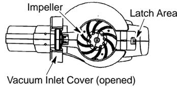
3. Turn the inlet restrictor counterclockwise and remove it from the unit. Do not close the inlet door. You will next attach the vacuum tubes.
