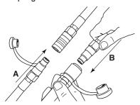
**CAUTION!** Two hose kits can be connected when hose lengths exceeding 18 m are required. Do not connect more than two kits as the couplings cause large power loss. See the Technical data.
