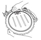
Fit the support roller guard and ensure that the flanges on the guide rollers still enter the blade's grooves correctly.
