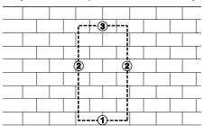
**CAUTION!** If the upper horizontal cut is made before the lower horizontal cut, the work piece will fall on the blade and jam it.
