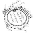
• Fit the support roller guard and ensure that the flanges on the guide rollers still enter the blade's grooves correctly. Now tighten the three screws fully.
