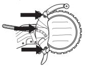
• Rotate the blade and make sure that the support rollers are not clamped against the blade.
