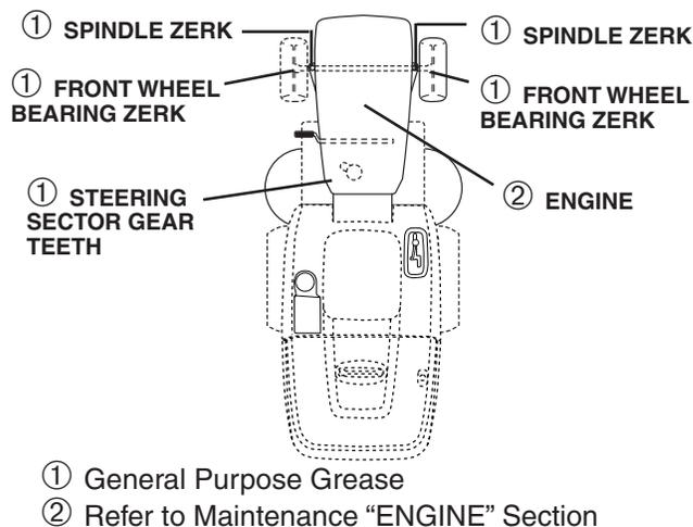
**IMPORTANT:** DO NOT OIL OR GREASE THE PIVOT POINTS WHICH HAVE SPECIAL NYLON BEARINGS. VISCOUS LUBRICANTS WILL ATTRACT DUST AND DIRT THAT WILL SHORTEN THE LIFE OF THE SELF-LUBRICATING BEARINGS. IF YOU FEEL THEY MUST BE LUBRICATED, USE ONLY A DRY, POWDERED GRAPHITE TYPE LUBRICANT SPARINGLY.
