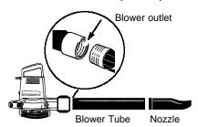
For Model 2695 only, the blower extension tube and nozzle are combined into one component.
