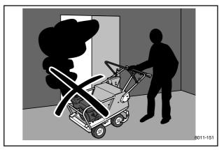
Do not use the machine indoors or in spaces lacking proper ventilation.
