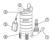
To ensure that the pump draws the water out, the water to be drained must be at least 10 cm deep.
