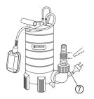
The universal fitting  $\ensuremath{ \ensuremath{ \bigcirc } }$  allows you to connect all the hoses listed in the previous table.
