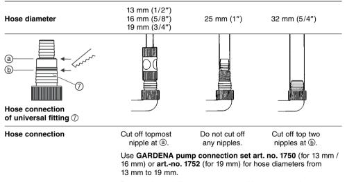
Best results in delivery capacity are achieved when using 32 mm (5/4") hoses.
