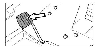
2. Carefully press down one of the pedals until the required speed is obtained.
