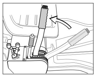
Lifting of the cutting unit
