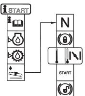
Starting instructions Read the instructions Check the engine's oil level Check the hydrostat's oil level Lift up the cutting unit Hydrostatic pedals in neutral position Brake If the engine is cold use the choke Start the engine Release the parking brake before driving
