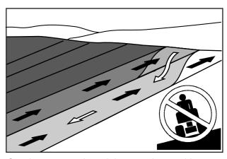
Cut slopes upwards and downwards, not sideways.
