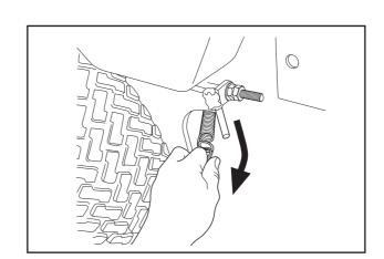
7. Place a foot on the front edge of the cutting unit near the wheel and raise the front edge of the unit to make it easier to remove the lift strut. Engage the strut in the holder.
