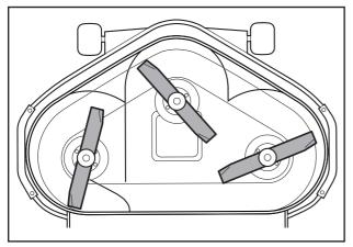
Cutting units with rear ejection
