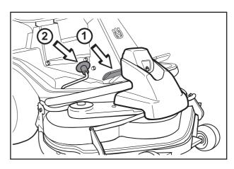
3. Push in the lock button on the lift lever and lower down the cutting unit.
