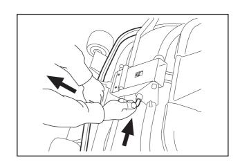
10. Grasp the front edge of the cutting unit, pull out and raise into the service position.
