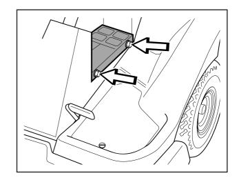
Pump the pedals and lubricate the moving parts using an oil can
