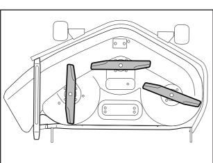
The blades should be balanced after sharpening.
