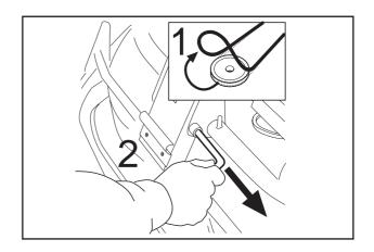
9. Pull the frame forwards and refit the pin.
