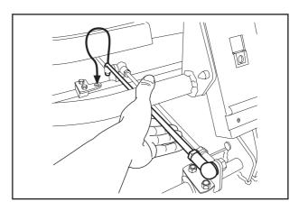
8. Lift off the drive belt (1). Then pull out the pin (2).
