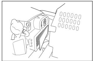
4. Unscrew the wing nut from the air filter and lift out the paper filter. Tap the filter against a hard surface to shake off the dust. If the paper filter is still dirty it should be replaced.
