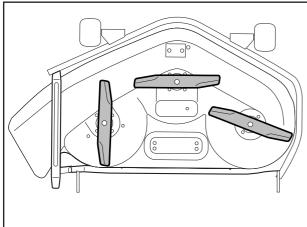
Cutting units with side ejection
