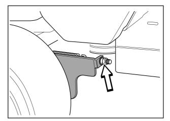
2. Adjust the unit's ground pressure by screwing in or out the adjusting screws located behind the front wheels on both sides.
