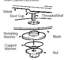
WARNING: Do notuse any blades, or fastening hardware other than the washersandnutsillustrated. These partsmust be provided by Weed Eater, and installed as shown below. Failure to use proper parts can causethebladetoflyoffandseriously hurtyou
