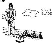
NOTE: If your unit has been assembled for trimmer headuse, refertothesection ATTACH-ING THE PLASTIC SHIELD ANDTRIMMER HEAD and reverse the steps to remove the plastic shield and trimmer head before you mount the metal shield and blade. Storethese parts for future use. Neveruse that immer head with the metal blade installed.
