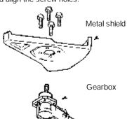
\$ Insert the 4 mounting screws through the bottom of the shield. Thread them into the gearbox. Tighten evenly and securely with one of the hex wrenches provided.
