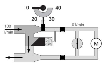
We can first study the function of the flow-rate selector. This is set at "0", the duct is closed and the full volume of fluid must be fed back to the return side. Flow from the pump presses the spring-loaded flow valve to the side and allows the fluid to pass under relatively low pressure.
