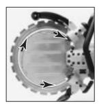
that it can be easily led out via the cutting groove. The U-shaped recess in the blade between the diamond segments serves as a transport channel for the water and the cut material's powder particles.
