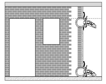
which will be entirely covered by the frame around the door or window. If the cut is made from two directions at the end points, overcut can be eliminated completely at cutting depths of up to 340 mm!
