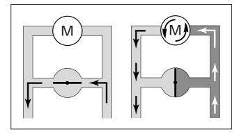
By leading some of the fluid directly to the return side, the flow to the tool can be varied. This principle is used for throttle control in Partner hydraulic cutters. When the machine is not operating, the entire flow passes virtually without pressure through the bypass valve. When the throttle control is pressed in, the bypass valve is closed and the hydraulic fluid is forced to pass through the motor.
