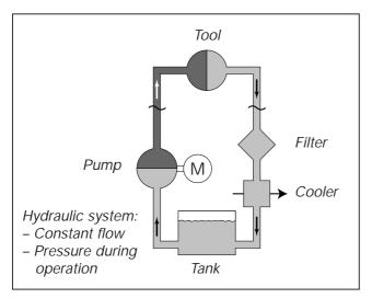
As we said earlier, a fluid cannot be compressed, which means that as long as the pump runs at a constant speed, the flow in the system is also constant, which is exactly the opposite of the compressed-air system.
