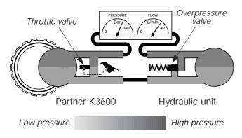
The pressure side of the hydraulic system is described by the upper half and the return by the lower half. As we shall see, there will be no change of pressure on the return side, only the flow path is changed under certain circumstances. That is why we only need to measure what happens on the pressure side, that is to say the side to which the hydraulic unit provides flow and pressure, and which drives the power cutter.
