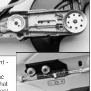
The machine is built for 16" cutting blades and the flange washers for the blade are rotation-inhibited to the spindle shaft, avoiding any tendency to self-tighten. The spindle shaft features easily replaceable centre bushings
