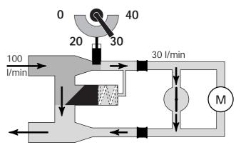
In the above figure, the flow-rate selector is set at 30 I/min. The inlet to the FC40 is partially restricted and most of the fluid passes through the flow valve directly to the return side.
