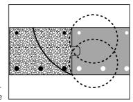
retained. The solid arch shows the cut that a centre-driven floor-cutter would make.
