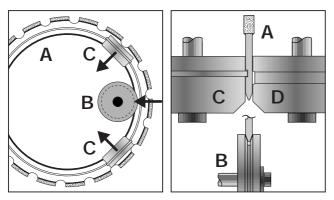
The unique concept behind the K3600 is the eccentric drive of the cutter blade. If the drive system had not given the machine such unique properties, then it would scarcely have made it to the market today. Eccentric drive in practical implementation has imposed considerable demands on development resources and is continuing to place major demands on day-to-day production.
