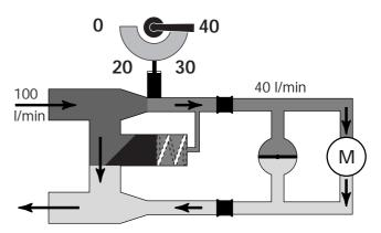
A Partner cutter is put to work (40 l/min). The pressure (resistance) increases in the supply line. This pressure is also led through the narrow duct to the rear of the flow valve, pushing it to the restricted setting. The higher the pressure in the feed line, the firmer the restriction and vice versa. Flow to the tool remains constant.
