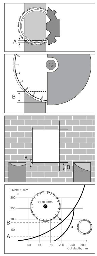
Wall thickness in the above examples is 200 mm. The two upper figures show overcut with the Partner K3600 and a centre-driven cutter (diameter 700 mm). The third figure shows the corresponding cuts as viewed by the operator and in cross-section.
