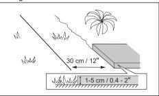
Put the boundary wire 10 cm / 4 in. (D) from an obstacle that is less than 1 cm / 0.4 in. high.
