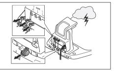
To reduce the risk of damage to electrical components in the product and the charging station, we recommend that all connections to the charging station are disconnected (power supply, boundary wire and guide wire) if there is a risk of a thunderstorm.
