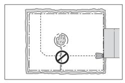
To make an island, isolate areas in the work area with the boundary wire. We recommend to isolate all stable objects in the work area.
