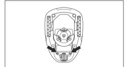
6. Release the latch of the connector (A) and pull it upwards.
