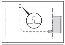
**Note:** Make a blueprint of the work area before you install the boundary wire and guide wire.
