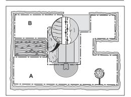
Put the boundary wire around the secondary area (B) to make an island. Refer to *To* make an island on page 19.
