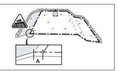
For slopes adjacent to a public road, put an obstacle of minimum 15 cm / 6 in. along the outer edge of the slope. You can use a wall or a fence as an obstacle.
