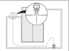
a) Put the 2 ends of the boundary wire and the end of the guide wire into the coupler.
