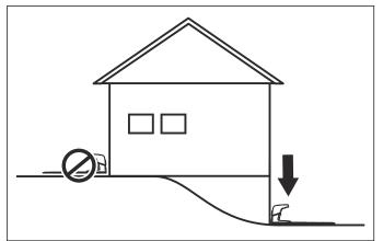
The charging station should not be placed on an island as this limits the laying of the guide wire in an optimal way. If the charging station has to be installed on an island, the guide wire also has to be connected to the island. Read more about islands in the *Boundaries within the working area on page 15*.
