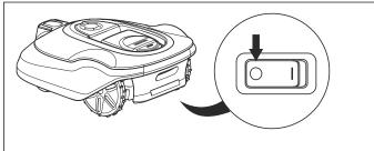
Always switch the robotic lawnmower off using the main switch if it requires maintenance or if the robotic lawnmower must be moved outside the working area.
