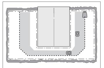
The factory settings can be used for many working areas, i.e. the robotic lawnmower itself can use the inbuilt functions to operate in the widest possible corridor. In more complex gardens e.g. where the guide wire is placed close to obstacles which cannot be isolated using the boundary loop, operational safety can be improved by carrying out some of the manual settings outlined below.
