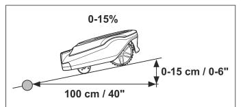
The boundary wire should not be laid across a slope that is steeper than 15%. There is a risk that the robotic lawnmower will find it difficult to turn there. The robotic lawnmower will then stop and the *Outside working area* fault message is displayed. The risk is at its greatest in damp weather conditions, as the wheels can slip on the wet grass.
