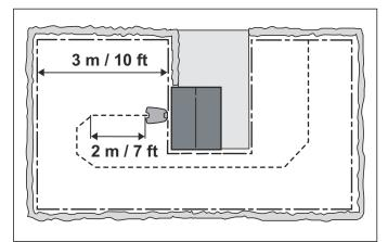
Do not put the charging station in confined spaces or in a corner. This can make it difficult for the robotic mower to find the charging station.
