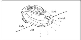
The **STOP** button on the top of the robotic lawnmower is mainly used to stop the robotic lawnmower when it's running. When the **STOP** button is pressed a hatch opens, behind which there is a control panel. The control panel is where you manage all the robotic lawnmower settings. The **STOP** button remains pressed in until the hatch is closed again. This together with the **START** button acts as a start inhibitor.
