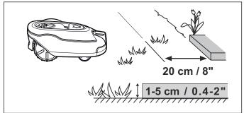
If the working area borders on a paving stone path or similar that is level with the lawn (+/- 1 cm), it is possible to allow the robotic lawnmower to run a little over the path. The boundary wire should then be laid 10 cm from the edge of the path. All the grass along the side of the paving stone path will be cut.
