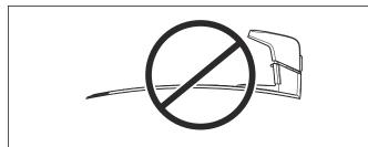
If the installation is done in a working area with a steep slope, the charging station should be placed at the bottom of the slope. This makes it easier for the robotic lawnmower to follow the guide wire to the charging station.
