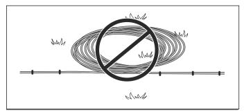
**WARNING:** Do not under any circumstances mount the power supply at a height where there is a risk it can be submerged in water (minimum 30 cm from the ground). It is not permitted to place the power supply on the ground.
