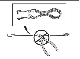
It is possible to let the low voltage cable cross the working area if it is stapled down or buried. The cutting height should be such that the blades can never come in contact with the low voltage cable.
