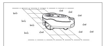
**CAUTION:** The robotic lawnmower must never run over gravel, mulch or similar material which can damage the blades.
