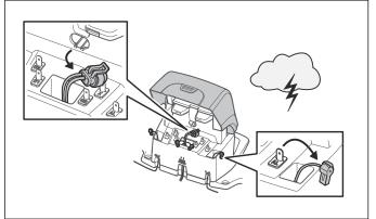
To reduce the risk of damage to electrical components in the robotic lawnmower and its charging station, we recommend that all connections to the charging station are disconnected (power supply, boundary wire and guide wires) if there is a risk of a thunderstorm.
