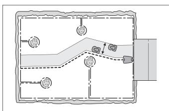
The aim of operating at varying distances from the wire is to reduce the risk of tracks forming. Therefore it is recommended to select the widest corridor possible allowed by the size of the working area.
