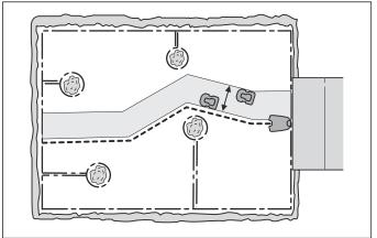
The robotic lawnmower runs at varying distances from the guide wire to reduce the risk of tracks forming. The area beside the wire which the robotic lawnmower then uses is called the Corridor. The wider the corridor allowed by the installation, the less the risk of tracks forming.
