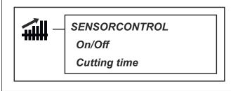
This function allows the robotic lawnmower to automatically adjust its mowing times based on how quickly the lawn grows. When the weather is good for grass growth, the robotic lawnmower mowes more often and when the grass growth is slower the robotic lawnmower will automatically spend less time on the lawn. The first mowing cycle of the day will however always be completed. After that, SensorControl will decide whether to continue or not.
