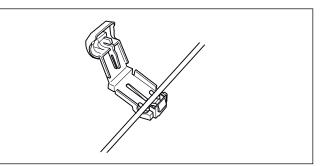
2. Press the connectors together using a pair of pliers. Press until you hear a click.
