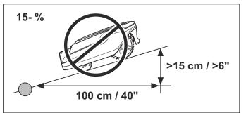
However, the boundary wire can be laid across a slope steeper than 15% if there is an obstacle that the robotic lawnmower is allowed to collide with, for example, a fence or a dense hedge.
