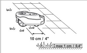
When the working area is divided by a paving stone path that is level with the lawn, it is possible to allow the robotic lawnmower to run over the path. It can be an advantage to lay the boundary wire under the paving stones. The boundary wire can also be laid in the joint between the paving stones. Ensure that the tiles are in level with the lawn to avoid excessive wear on the robotic lawnmower.
