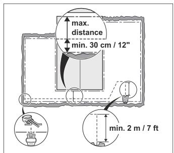
The guide wire, as the boundary wire, can be stapled to or buried in the ground.
