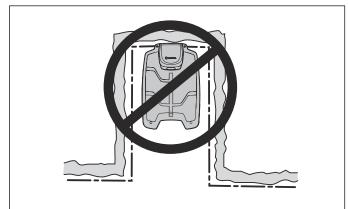
The charging station must be positioned on relatively level ground. The front end of the charging station cannot be positioned higher or lower than the back end according to picture below.
