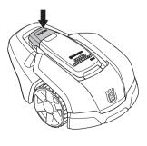
The control panel on the top of the robotic lawnmower is where you manage all the robotic lawnmower settings. Open the control panel cover by pressing down the **STOP** button.
