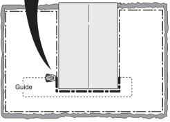
4. a) Assume that the indicator lamp flashed yellow in test a) above. Reset all connections to their original positions. Then disconnect AR. Connect a new loop wire to AR. Connect the other end of this new loop wire somewhere at the centre of the installation.
