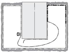
5. When the break is found, the damaged section must be replaced with a new wire. The damaged section can be cut out if it is possible to shorten the boundary wire. Always use original couplers.
