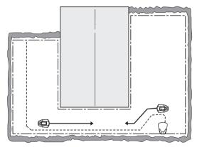
In the passage, the guide wire must therefore be placed so that the robotic lawnmower has as much space to run in as possible. The distance between the boundary loop and the guide wire must however be at least 12" (30 cm).
