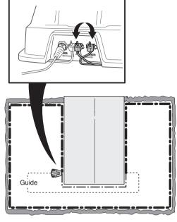
b) Put AL and Guide back in their original positions. Then switch AR and Guide. If the indicator lamp flashes yellow, then the break is somewhere on the boundary wire between AR and the point where the guide wire is connected to the boundary wire (thick black line in the illustration). 3018-05
